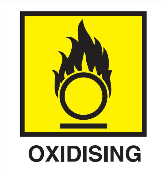
Figure 4: Label on oxidising materials
